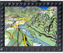
... with MT TAWS - Terrain details in high resolution alert you about the dangers of collision – clearly and with color codes always in relation to your flight altitude
