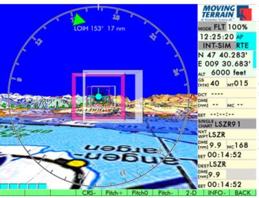
The flight path indicator anticipates the position of the aircraft related to 10 sec. continuation. The aircraft symbol anticipates exactly the required fligh path including wind influences and WCA's.
